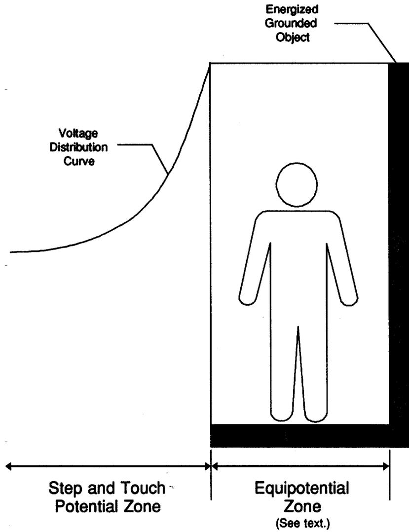
**Figure 3 - Protection from Ground-Potential Gradients**
