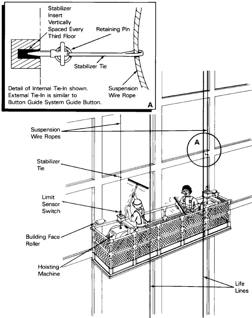
Figure 3. Typical Self-Powered Platform--
