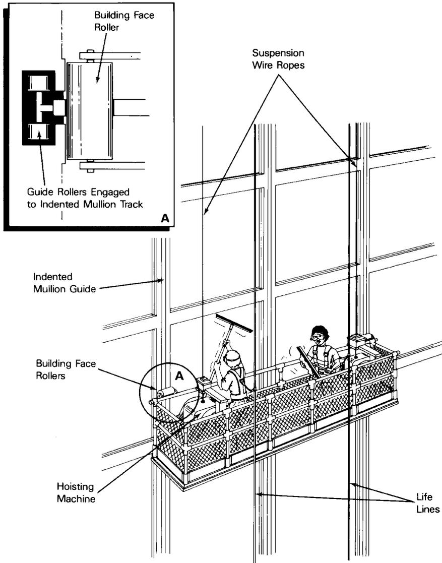
Figure 2. Typical Self-Powered Platform--
